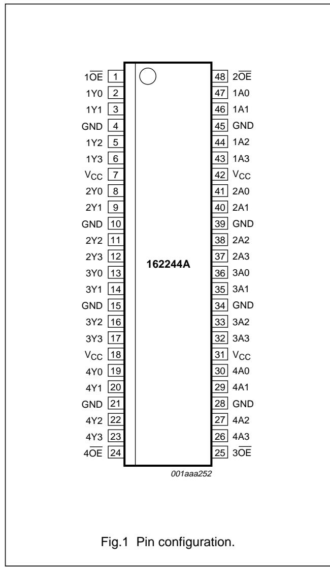
Fig.1 Pin configuration.
