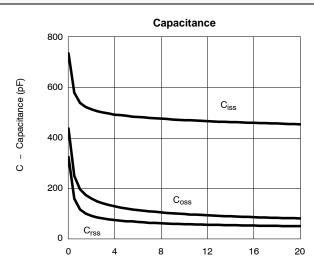
V<sub>DS</sub> - Drain-to-Source Voltage (V)
