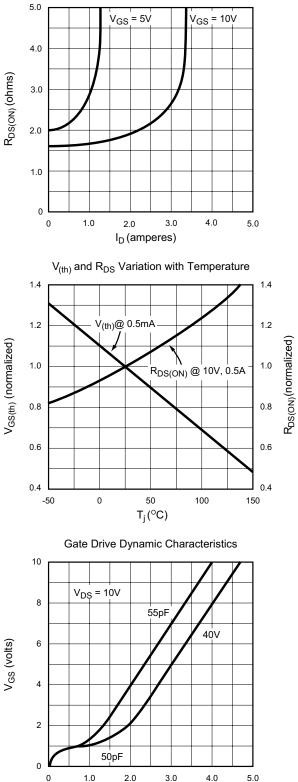
On-Resistance vs. Drain Current
