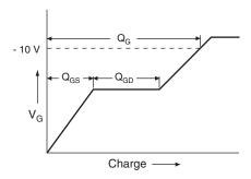
Fig. 13a - Basic Gate Charge Waveform
