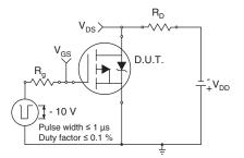
Fig. 10a - Switching Time Test Circuit
