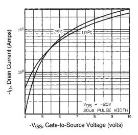
Fig. 3 - Typical Transfer Characteristics
