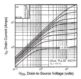
Fig. 2 - Typical Output Characteristics,  $T_A$  = 175 °C
