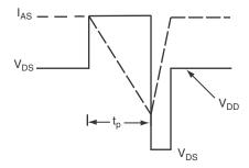
Fig. 12b - Unclamped Inductive Waveforms
