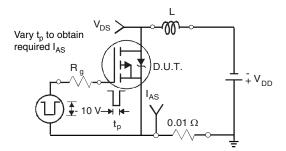
Fig. 12a - Unclamped Inductive Test Circuit
