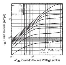
Fig. 1 - Typical Output Characteristics, T<sub>A</sub> = 25 °C
