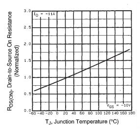
Fig. 4 - Normalized On-Resistance vs. Temperature
