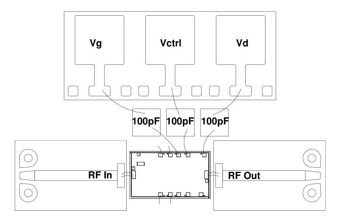
All DC connections may be brought in from either side of the chip (Use Pad 4 or 10, Pad 5 or 9, and Pad 6 or 8) 0.01uF external Caps are recommended on Drain, Gate line, 10 ohm external series R between 100pF cap and 0.01uF cap is recommended for Gate line Source connections (Pad 2, 3, 11, 12) are bonded to ground. All four bond wires are required for stability.
