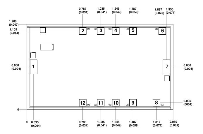
Units: millimeters (inches) Thickness: 0.100 (0.004)
