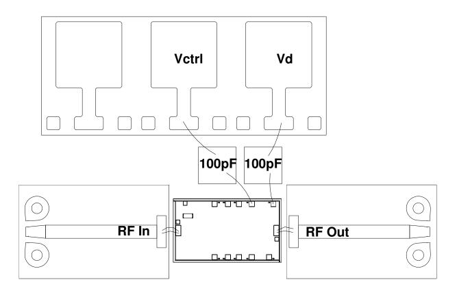
All DC connections may be brought in from either side of the chip (Use Pad 5 or 9, and Pad 6 or 8) 0.01uF external Caps are recommended on Drain line
