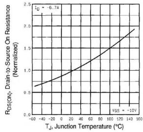
Fig. 4 - Normalized On-Resistance vs. Temperature
