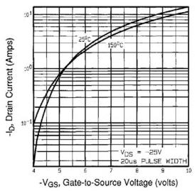
Fig. 3 - Typical Transfer Characteristics
