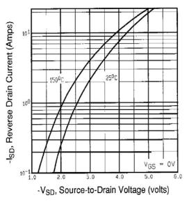
Fig. 7 - Typical Source-Drain Diode Forward Voltage
