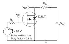
Fig. 10a - Switching Time Test Circuit
