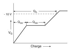
Fig. 13a - Basic Gate Charge Waveform
