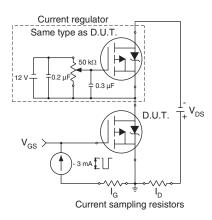
Fig. 13b - Gate Charge Test Circuit
