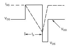
Fig. 12b - Unclamped Inductive Waveforms
