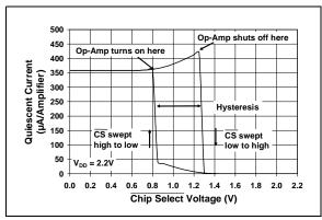
FIGURE 2-21: Quiescent Current vs. Chip Select (CS) Voltage at  $V_{DD} = 2.2V$  (MCP6283 and MCP6285 only).
