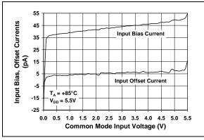
**FIGURE 2-9:** Input Bias, Offset Currents vs. Common Mode Input Voltage at  $T_A = +85$ °C.
