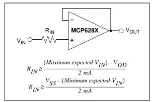
**FIGURE 4-2:** Input Current Limiting Resistor  $(R_{IN})$ .
