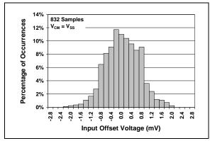
FIGURE 2-1: Input Offset Voltage.
