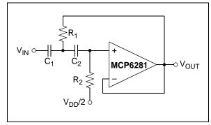
FIGURE 4-7: Sallen-Key High-Pass Filter.
