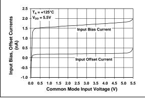
**FIGURE 2-12:** Input Bias, Offset Currents vs. Common Mode Input Voltage at  $T_A = +125$ °C.
