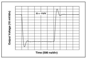
**FIGURE 2-29:** Small-Signal, Inverting Pulse Response.
