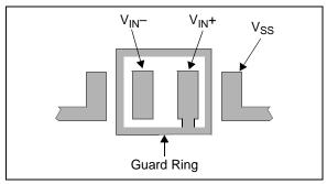
**FIGURE 4-6:** Example Guard Ring Layout for Inverting Gain.
