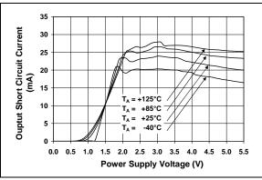
**FIGURE 2-20:** Output Short Circuit Current vs. Power Supply Voltage.
