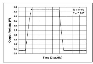
**FIGURE 2-25:** Large-Signal, Non-inverting Pulse Response.
