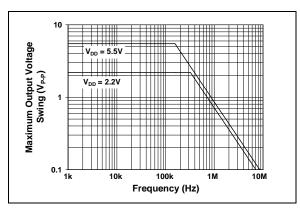
**FIGURE 2-15:** Maximum Output Voltage Swing vs. Frequency.
