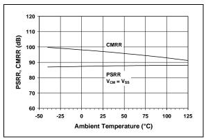
**FIGURE 2-11:** CMRR, PSRR vs. Ambient Temperature.
