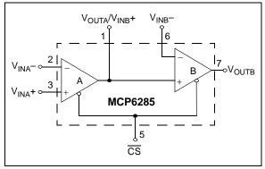
FIGURE 4-5: Cascaded Gain Amplifier.
