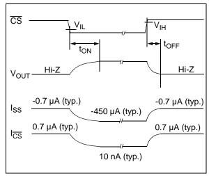
FIGURE 1-1: Timing Diagram for the Chip Select (CS) pin on the MCP6283 and MCP6285.
