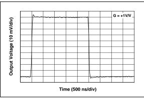
**FIGURE 2-26:** Small-Signal, Non-inverting Pulse Response.
