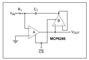
FIGURE 4-13: Integrator Circuit with Active Compensation.
