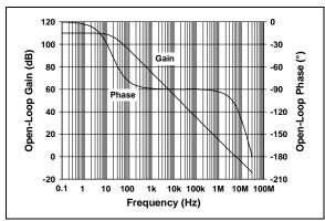
**FIGURE 2-14:** Open-Loop Gain, Phase vs. Frequency.
