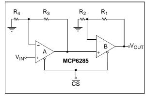
FIGURE 4-10: Cascaded Gain Circuit Configuration.
