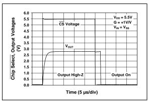
**FIGURE 2-30:** Chip Select  $\overline{(CS)}$  to Amplifier Output Response Time at  $V_{DD} = 5.5V$  (MCP6283 and MCP6285 only).
