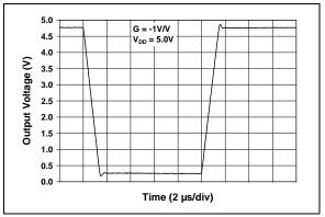
**FIGURE 2-28:** Large-Signal, Inverting Pulse Response.
