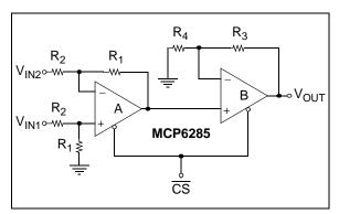
FIGURE 4-11: Difference Amplifier Circuit.
