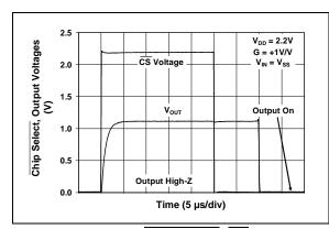
**FIGURE 2-27:** Chip Select  $(\overline{CS})$  to Amplifier Output Response Time at  $V_{DD} = 2.2V$  (MCP6283 and MCP6285 only).
