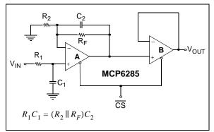
FIGURE 4-12: Buffered Non-inverting Integrator with Chip Select.
