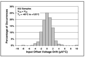
FIGURE 2-4: Input Offset Voltage Drift.
