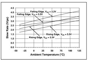
**FIGURE 2-18:** Slew Rate vs. Ambient Temperature.
