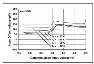
**FIGURE 2-3:** Input Offset Voltage vs. Common Mode Input Voltage at  $V_{DD} = 2.2V$ .
