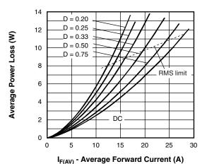
Fig. 6 - Forward Power Loss Characteristics
