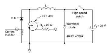
Fig. 8 - Unclamped Inductive Test Circuit
