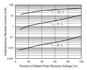
Figure 4. Typical Reverse Characteristics
