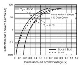
Figure 3. Typical Instantaneous Forward Characteristics
