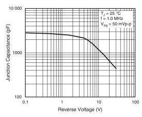
Figure 5. Typical Junction Capacitance
