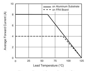
Figure 1. Forward Current Derating Curve
