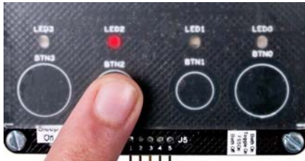
1. Touch a button; LED turns on
