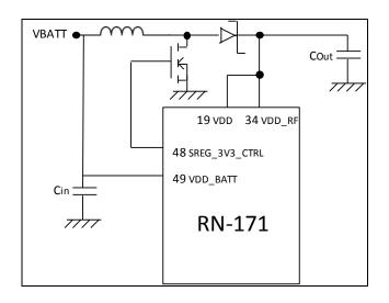
Designs that include the boost regulator will provide good supply to the flash even when the battery voltage drops close to 1.8V.
