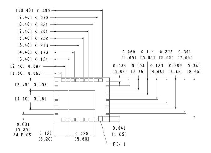
The nominal size of the part is 12x9.5mm with a height of 1.7mm
