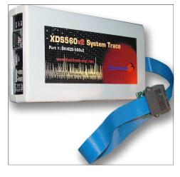
ribbon coax JTAG cable. The XDS560v2 adds support for IEEE1149.7 and the system trace module (STM), an interface on the TI heterogeneous multi-core (ARM + DSP) devices. If you are familiar with the Blackhawk LAN560 product, you will already be familiar with this new design.
