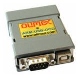
ARM-USB-OCD is unique device which combine JTAG debugging hardware, RS232 virtual port and power supply adapter in one single compact form. Many of the new laptop computers have no parallel nor serial ports but only USB, with ARM-USB-OCD you can debug your ARM boards, have full featured virtual RS232 port with all modem signals on it and the power jack can provide three fixed value voltages 5V – 9V – 12V DC via jumper selection.
