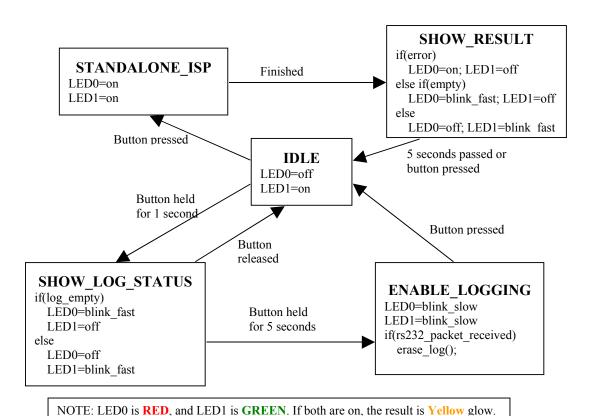
In case of autonomous operation error, the RED LED will blink for a while. The number of flashes indicates the error that caused the failure. Error codes are given in the table below.
