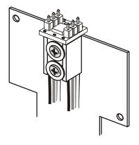
**Step 1:** Mount the HM55B Compass Module on the back side of the PING))) Mounting Bracket using (2) 4/40<sup>1/2</sup>" screws, (2) 4/40 nuts and (2) 10" servo extension cables.
