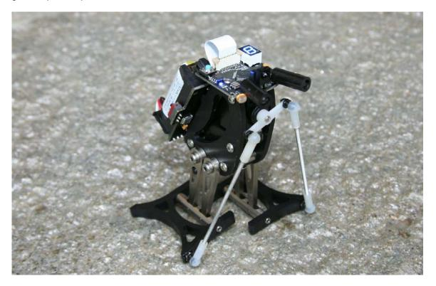
The Penguin's microcontroller is an embedded BASIC Stamp2px24 module, the fastest and most powerful BASIC Stamp in the Parallax lineup. The Penguin requires three hours to assemble, after which it is a PBASIC programming challenge to exploit all of the robot's capabilities.
