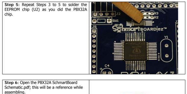
Each of the parts that you will install from here out will need the appropriate portions of solder and flux; depending on the type of solder you use will determine the heat needed for the soldering iron; please see solder package for details. The SchmartBoard uses lead-free solder and is suggested as the type to use.
