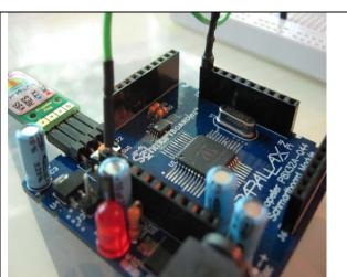
Step 16: Run this test code that blinks the LED on I/O pin P23 to confirm operation. Change the Pin constant and circuit to test the rest of the I/O pins.
