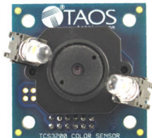
TCS3200-DB with lens, standoffs, and screws.
