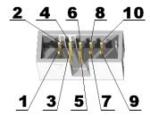
This connector allows programming and debugging via AVR-JTAG or other compatible tools.
