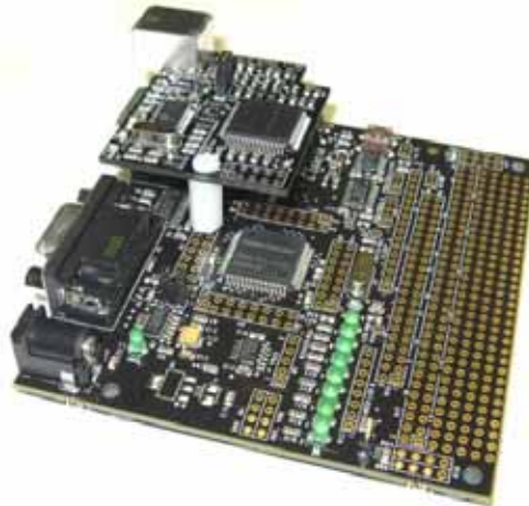
Figure 4: Installing the VJTAG-USB on the devboard
