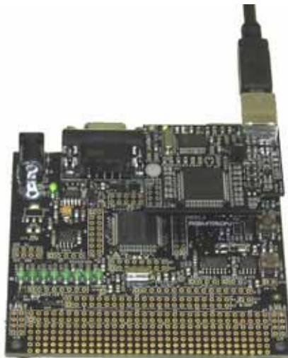
Figure 5: Connecting the USB cable to the VJTAG-USB
