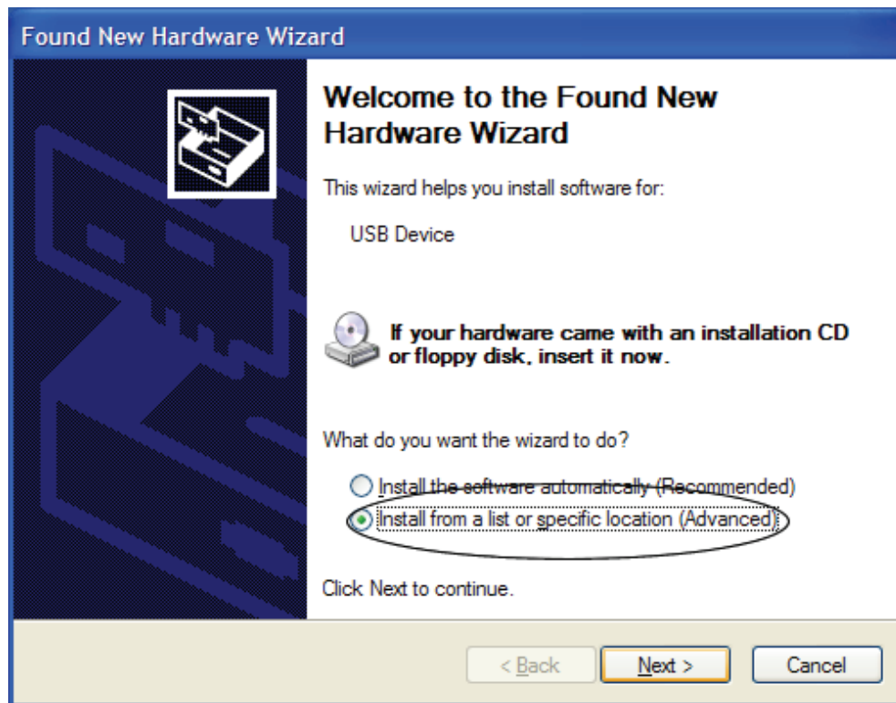
Figure 6. USBXpress Driver Installation for Windows XP—Options
