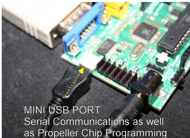
Figure 15.48 – The Mini-USB port on the Chameleon connects to the FTDI USB to Serial converter chip.
