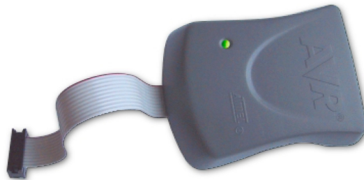
Figure 4.1 – The Atmel AVR ISP MKII programmer.
