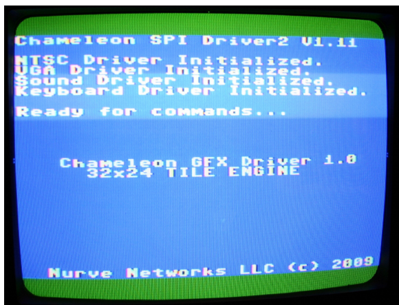
Figure 15.68 – The NTSC and VGA monitors showing the Chameleon AVR's output after installing the Propeller driver firmware.
