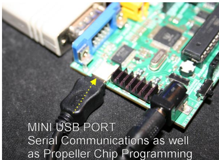
Figure 15.51 – The Mini-USB port on the Chameleon connects to the FTDI USB to Serial converter chip.
