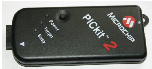
Figure 4.1 – The Microchip PICKit 2 programmer.
