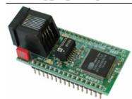
CS8900A-H is low cost development board with the popular Cirrus Logic CS8900A-CQ3 Ethernet controller. It allow easy to interface any microcontroller with 8 and 16 bit width data bus width, and support both polling and interrupts.
