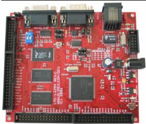
LPC-L2294 is compact development board with LPC2294 ARM7DTMI microcontroller from Philips Semiconductors Inc. with 512KB internal flash, 64KB internal RAM, There are two options:1MB external RAM + 2MB external Flash and 8MB external RAM + 4 MB external Flash.
