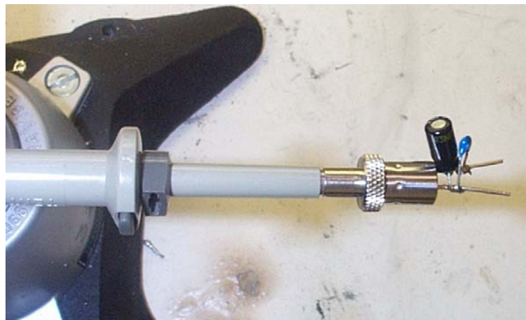
Figure 46 – Oscilloscope Probe with Probe Master ( www.probemaster.com ) 4987A BNC Adapter. (Modified with wires for ripple measurement, and two parallel decoupling capacitors added)
