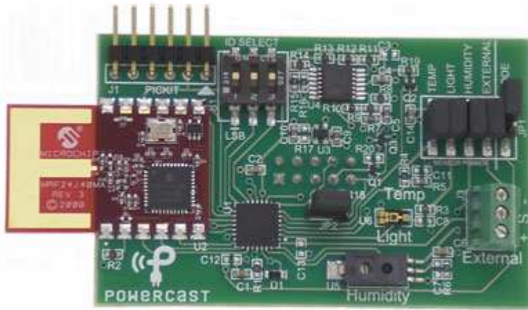
WSN-EVAL-01 wireless sensor board
