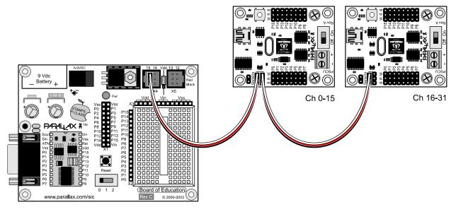
Note: Networking/Daisy-chaining of PSCU modules is not supported when using a USB connection. For USB control you will need a separate USB port for each unit and all units will be set to Port Mode 0.
