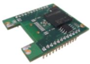
XPort Direct+ is also offered without an RJ45 connector. The XPort Direct+ NC (no connector) is a lower-priced option enabling you to place the connector anywhere on the board, based on your design requirements.
