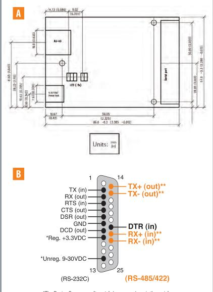
\*The Device Server can alternately be powered up via the serial port using one of these pins.
