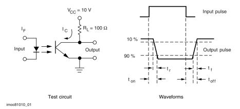
Fig. 7 - Switching Time Test Circuit and Waveforms
