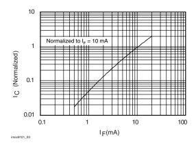
Fig. 2 - Collector Current vs. LED Forward Current
