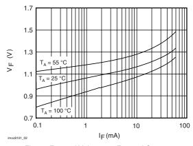
Fig. 1 - Forward Voltage vs. Forward Current
