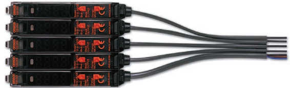
The E3X-DA-S requires three wiring connections for the master sensor only. Each additional sensor in a group requires only one wiring connection. Shown: ONLY 7 WIRES with no additional extension connectors.
