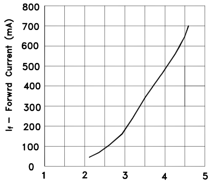
VF-Forward Voltage (V) Forward current vs. Forward voltage
