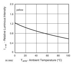
Figure 8. Rel. Luminous Intensity vs. Ambient Temperature
