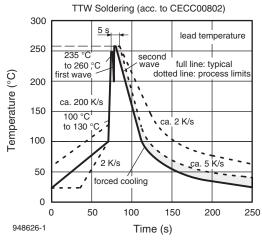
Figure 13. Double Wave Soldering of Opto Devices (all Packages)
