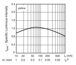
Figure 7. Rel. Lumin. Intensity vs. Forw. Current/Duty Cycle
