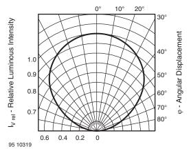
Figure 3. Rel. Luminous Intensity vs. Angular Displacement
