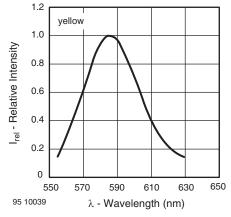
Figure 4. Relative Luminous Intensity vs. Wavelength
