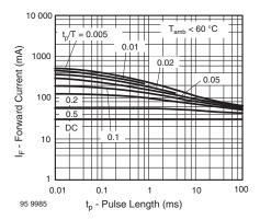
Figure 2. Forward Current vs. Pulse Length
