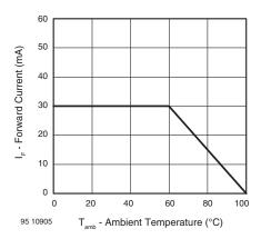
Figure 1. Forward Current vs. Ambient Temperature
