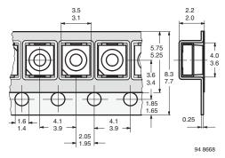
Figure 9. Tape Dimensions in mm for PLCC-2
