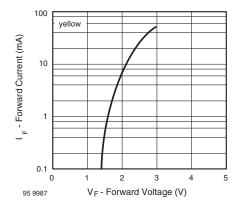
Figure 5. Forward Current vs. Forward Voltage
