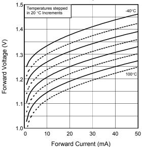
Forward Voltage vs. Forward Current vs. Temperature
