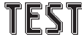
Overlaying (EXOR) of the "outline font" at pos. 2,2. results in an "outline font with fill"
