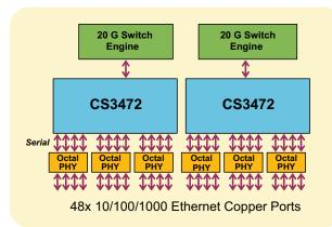
Serial SGMII connections to Copper PHY's allow use of new high-density PHY's and reduce board complexity. Direct connection to SFP optics is also supported.
