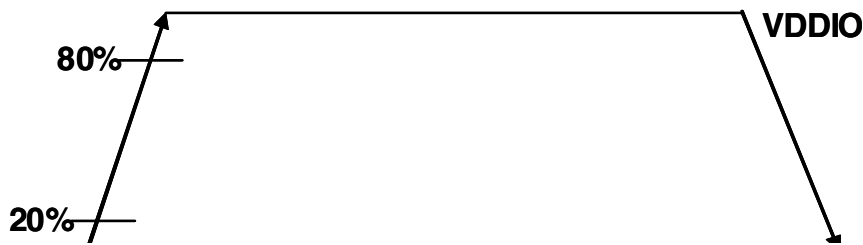
Figure 4. Output Pad Transition Waveform
