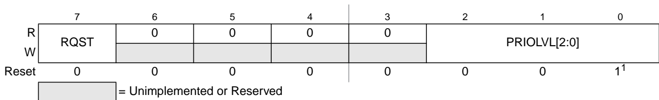
Figure 16-13. Interrupt Request Configuration Data Register 7 (INT_CFDATA7)
