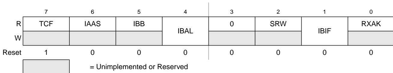
Figure 9-7. IIC Bus Status Register (IBSR)
