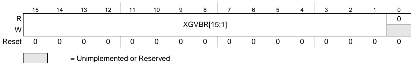
Figure 6-5. XGATE Vector Base Address Register (XGVBR)
