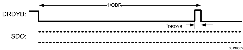
FIGURE 19. DRDYB Behavior for an Incomplete ADC_DOUT Reading
