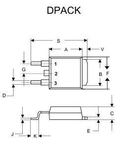
PIN 1. BASE PIN 2. COLLECTOR PIN 3. EMITTER
