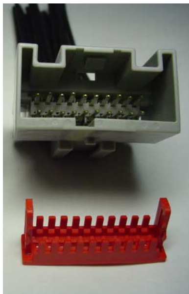
Un-damaged TPA after removal
