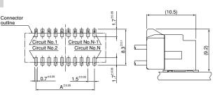
Note: 1. Tolerances are non-cumulative: ±0.05mm for all centers. 2. The dimensions above should serve as a guideline. Contact JST for details.
