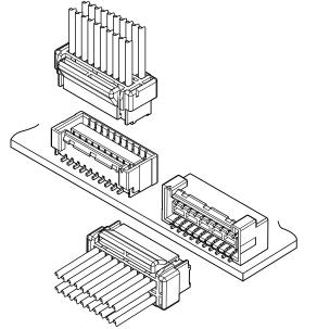
In order to correspond to the high-density PC board designing, this ZPD connector is designed as 1.5mm pitch double row type connector with secure locking device. Low insertion force is realized and good mating feeling is also prepared, and these provide the certain mating operation.
