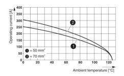
Derating diagram (3 modules in HC-B 24 housing)
