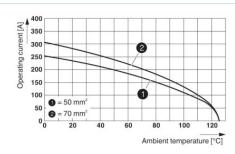
Derating diagram (3 modules in HC-B 24 housing)
