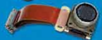
Fiber Optic MT Ferrule Termini in 38999 Connectors
