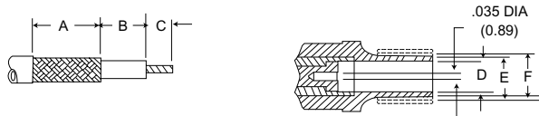
50 Ohm Contact (RG-196U) (assembly steps 1, 2, 3, 4, 5 & 8)
