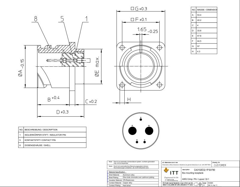
Contact Material: Copper alloy Contact Plating: Hard silver
