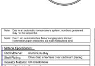
Contact Material: Copper alloy Contact Plating: Hard silver
